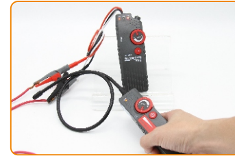
Tracing Electricity Cable
